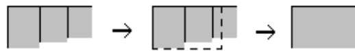
Figure 10: The process of combining components of a region to a single piece.
