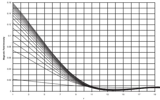
Figure 1: The behavior of magnetic field (from model in section 6.1) against  $r$  at different depth  $z = 0, 0.2, 0.4, \dots, 3.2, 3.4m$ .
