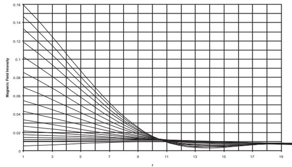
Figure 2: The behavior of magnetic field (from model in section 6.2) against  $r$  at different depth  $z = 0, 0.2, 0.4, \dots, 3.2, 3.4m$ .
