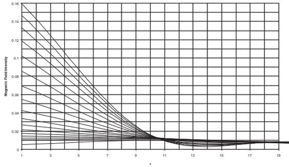
Figure 3: The behavior of magnetic field (from model in section 6.3) against  $r$  at different depth  $z = 0, 0.2, 0.4, \dots, 3.2, 3.4m$ .
