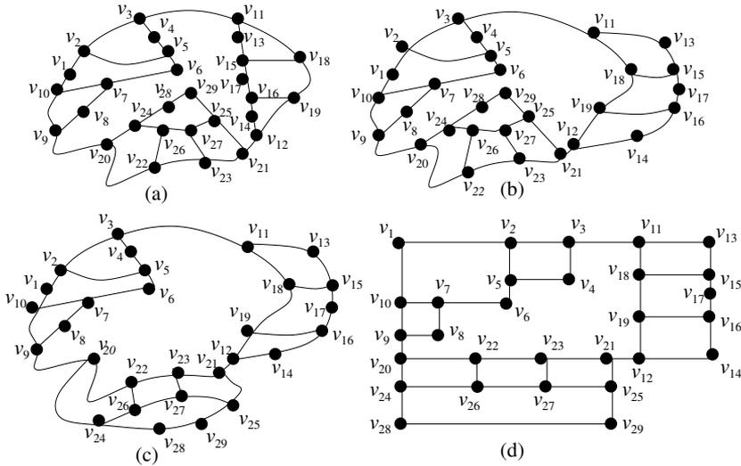
FIGURE 3. (a)-(b) Two plane embeddings of a planar graph  $G$  which have no rectilinear orthogonally convex drawing, (c) a planar embedding  $\Gamma$  of  $G$  which has a rectilinear orthogonally convex drawing, and (d) a rectilinear orthogonally convex drawing of  $\Gamma$ .
