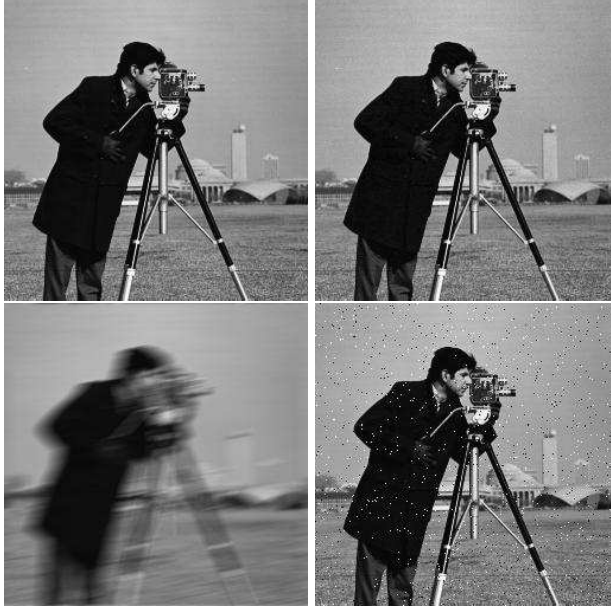
FIGURE 1. Main image (top left), degraded image (top right) with MSE= 15.0742, PSNR= 36.3485, SNR= 30.7657, SSIM= 0.9501, the motion blurred image (bottom left) with MSE= 770.5704, PSNR= 19.2627, SNR= 13.6800, SSIM= 0.6138 and the salt & pepper blurred image (bottom left) with MSE= 434.2821, PSNR= 21.7531, SNR= 16.1704, SSIM= 0.5690.
