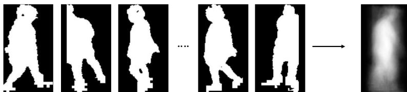
FIGURE 1. Example of a GEI generated from a walk with the viewpoint issue.
