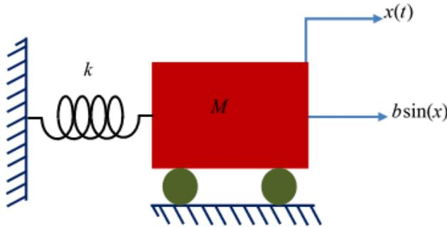
FIGURE 1. Geometric Structure of the Problem.
