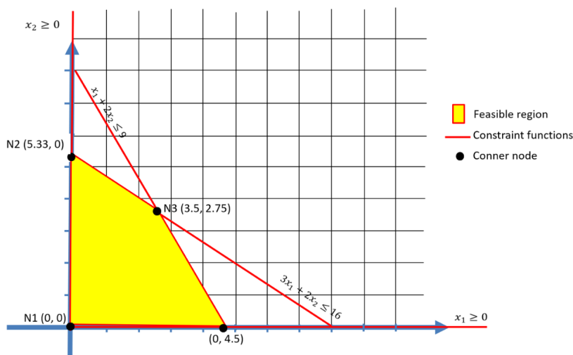
FIGURE 5. The feasible region of the example from the graph method.
