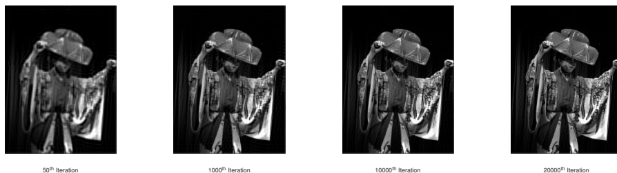
FIGURE 4. The reconstructed images being 50th, 1000th, 10000th and 20000th used iterations of the Gaussian blurred image on Figure 3.
