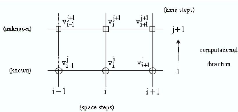
Figure 3 : Schematic form of the Crank-Nicolson method.
