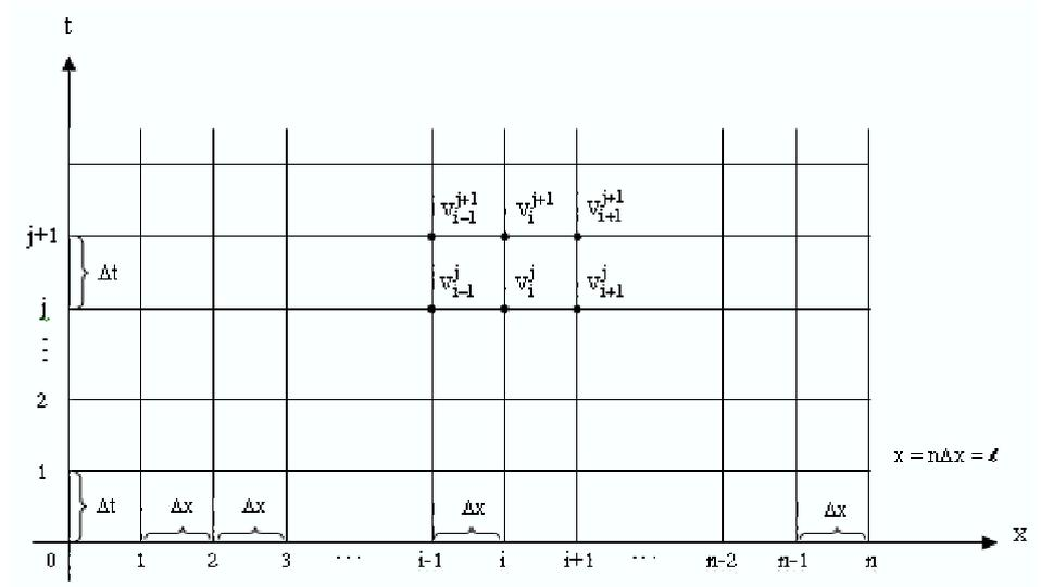
Figure 1 : Subdivision of the domain into intervals of  $\Delta x$  and  $\Delta t$  for finite-difference representation of the one-dimensional, time-dependent heat conduction equation.
