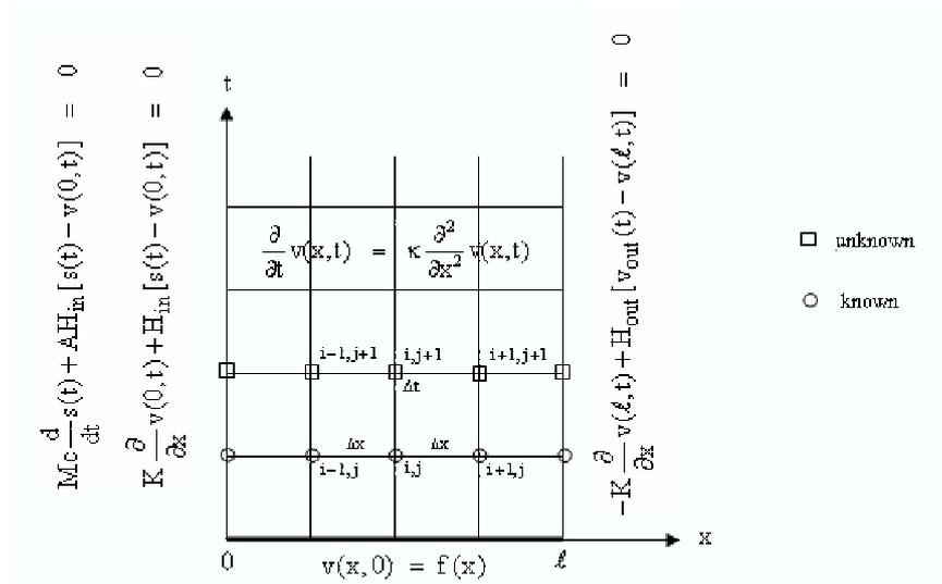
Figure 5 : Boundary condition and values needed for computation at time  $j + 1$  .
